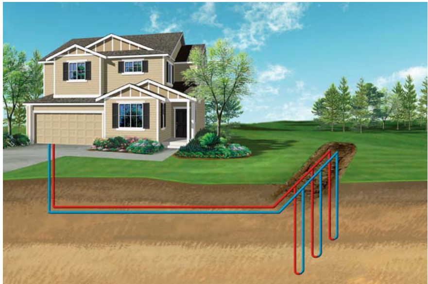
Figure 5: AN EXAMPLE OF VERTICAL CLOSED LOOP SYSTEM 6
