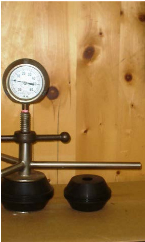
FIGURE 12-4: FLOWING WELL PRESSURE GAUGE DEVICE
