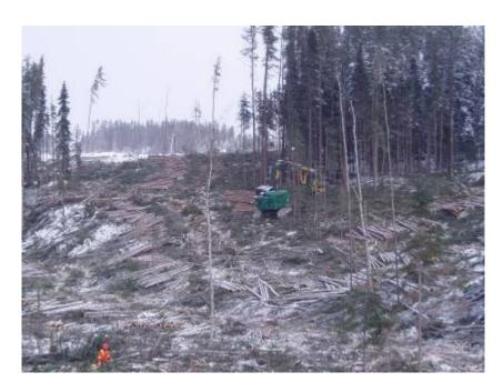
Figure 5.2h. A cut-to-length harvester can be used to de-limb and slash trees at the stump to avoid moving nutrients associated with unutilized fibre to roadside (photo by Mike Curran).
