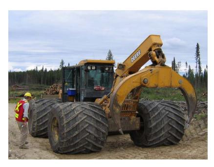
Figure 5.2j. Using machinery with low ground pressure options, such as these high floatation tires, can help to minimize damage and may expand the range of sites on which operations can occur in unfrozen conditions (photo by Joe Maure).
