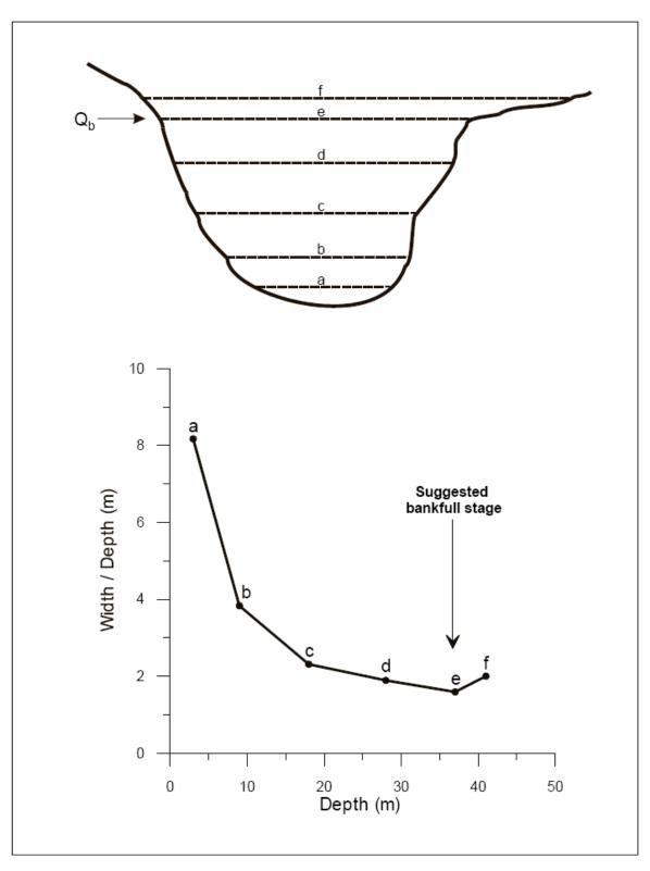
Figure 3 Determining bankfull stage using the width/depth ratio (from Wolman 1955; Knighton 1998).
