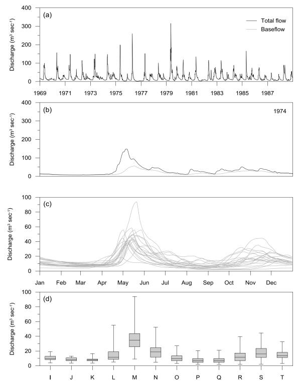
**Figure 4** The continuous baseflow separation process and calculation of indicators showing: a) continuous baseflow separation versus total flow using the reference condition period of record; b) one calendar year of data illustrating the baseflow separation; c) daily baseflow hydrographs for the period of record; d) monthly baseflow box plots showing the interquartile range (IQR) (shaded box) and one step from the IQR (whiskers – also referred to as the upper and lower adjacent values).
