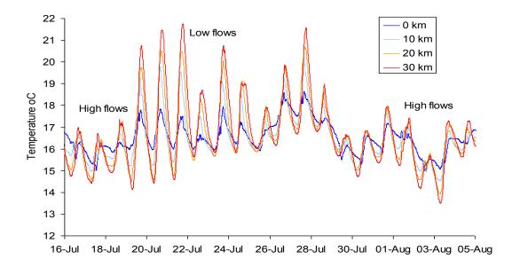
**Figure 2.** An example of how water begins to increase in temperature downstream from a metalimnetic release dam over a distance of 30 km. High flows during peaking take longer to warm than low flows.
