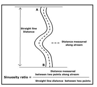
**Figure 2**. Method for calculating sinuosity index (SI) (Source: Ritter, 2006).
