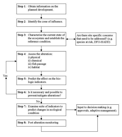
**Figure 2** Schematic diagram of the process of assessing the level of alteration resulting from in-stream development, predicting the potential changes to ecological condition of the river system and monitoring the ecological condition following alteration.
