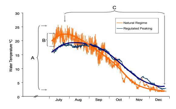
**Figure 1.** Bottom-draw dams in thermally stratified reservoirs tend to increase temperatures in winter, lower them in summer, fluctuate less diurnally and seasonally, and exhibit seasonally displaced maxima. Indicators that reflect these differences in thermal regimes include (A) reduction in annual temperature range, (B) reduction in daily temperature range, and (C) phase shift in annual temperature extremes and cooling/warming timing and rates of change.
