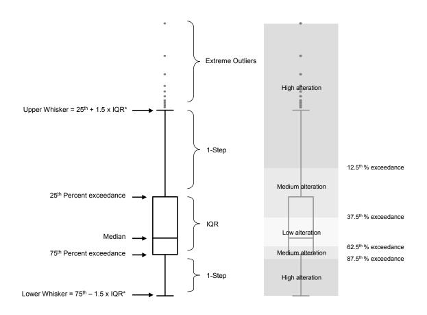
**Figure 3** Anatomy of a box plot and how it is used to assess alteration. Measures of dispersion around the median are shown as percent exceedances, a common convention in hydrology when analysing flow duration curves (FDCs).
