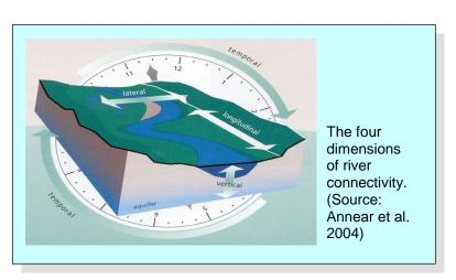
downstream connection within the river, the lateral dimension refers to the river's connection to the riparian and floodplain areas, the vertical dimension refers to the connection between surface and groundwater, the hyporheic zone of the river bed, and finally the temporal dimension refers to the change over time in the relative importance of different river processes (Ward 1989).
