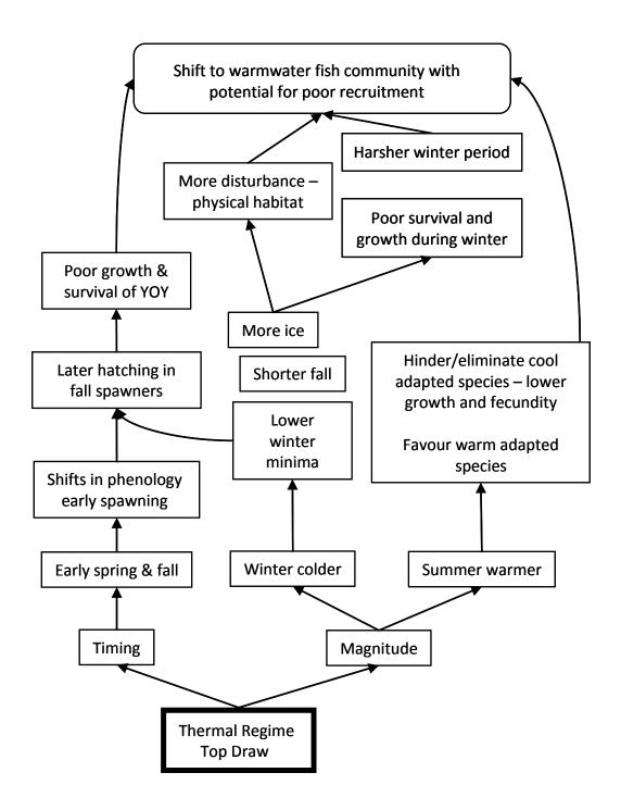
Figure 4. Possible effects of a top-draw dam on thermal regime and fishes in a cold water river.
