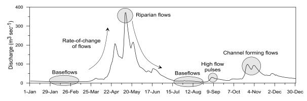
**Figure 1** Ecologically important flow components, used to assess hydrologic alteration, identified on an annual hydrograph.
