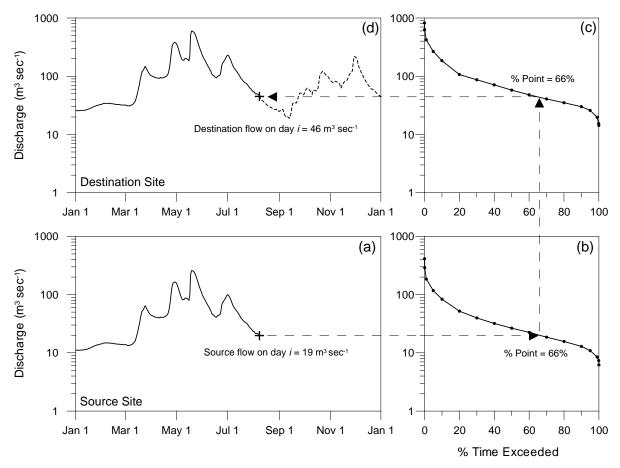
**Figure 2.** Streamflow generation procedure using (a) an observed hydrograph and (b) position of a daily mean flow on its FDC to (c) find the discharge value associated with the same percentage point on the destination site FDC to (d) create the simulated hydrograph for the destination site (Source: Metcalfe *et. al.* 2005a).
